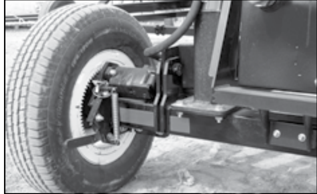
Fig 88 - Bin fill conveyor drive wheel
