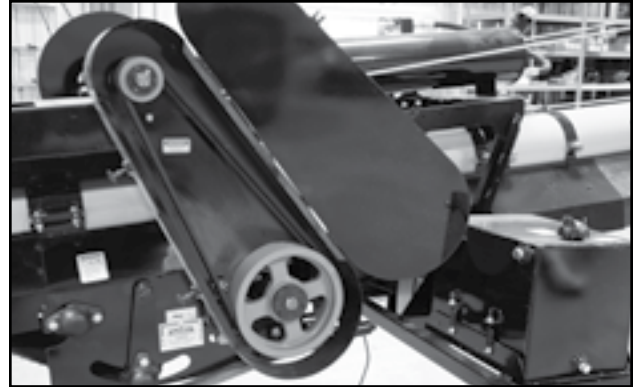
Fig 81 - Belt drive with guard opened
