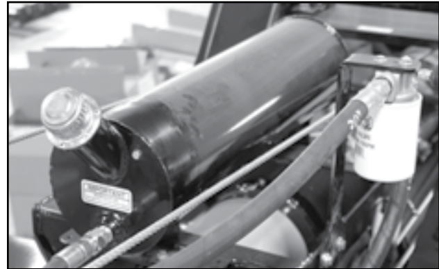
Fig 61 - Hydraulic system filter
