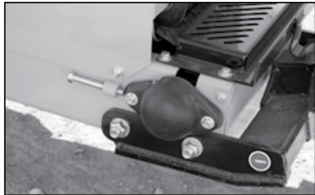
Fig 53 - Adjustment bolts on hopper
